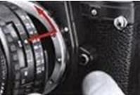
3. Seat the lens on top of the camera body's lens mounting flange 1, making sure the lens mounting index 12 is aligned with the aperture/distance scale index 19. Then twist the lens by its mounting ring 18 until it clicks and locks into place.
