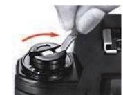
**6.** Rotate film rewind crank **24** take up film slack. Be careful that you do not wind film back into the cassette.
