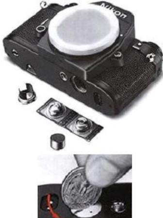
**1.** Unlock the battery chamber lid **46** with a coin.
