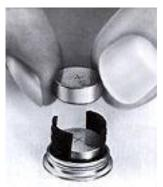
**3.** Insert the battery (batteries), with the "+" sign(s) facing up, into battery clip.
