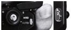
7. Advance the film, press the shutter release button and advance the film again until the frame counter 1 indicates "1" to start AUTO operation.
