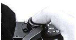
9. Press shutter release button 3 all the way. *Note:* Do not attempt to take pictures prior to frame 1, the start of **AUTO** operation.
