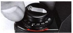
7. Snap camera back closed, then set ASA by lifting up and turning ASA film speed selector ring *26*.
