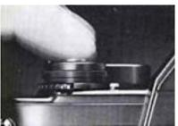
1. Depress the shutter release button 3 with steady, even pressure.
