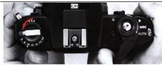
**11.** Confirm film advance: film rewind knob **25** turns opposite engraved arrow as winding lever is stroked.
