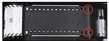
**5.** Load film. To ensure proper film winding, make sure that both edges of the film engage the film sprockets *37*.
