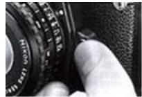
4. To remove the lens: Press the camera's lens release button (3), and twist the lens clockwise by its mounting ring until it becomes loose.
