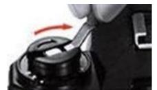
**2.** Turn the film rewind crank *24* in the direction of the engraved arrow with even pressure until rewind "tension" gets lighter.
